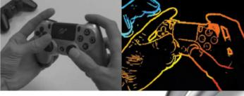
**Topaz5D™** is a 1,920 x 1,080 resolution, low noise global shutter 2D and 3D image sensor, designed with Teledyne e2v's proprietary CMOS technology and specific 3D post-processing optical layers. This delivers uncompromised 2D and 3D data in parallel, ideal for multiple logistics, robotic guidance, AR/VR tracking and anti-spoofing applications.
